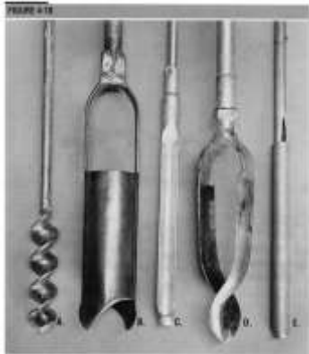
FIGURE 4-18 Sediment augers and tubes. A, screw-in worm auger; B, barrel auger; C, sampling tube; D, "Baker" type auger; E, post sampler.
